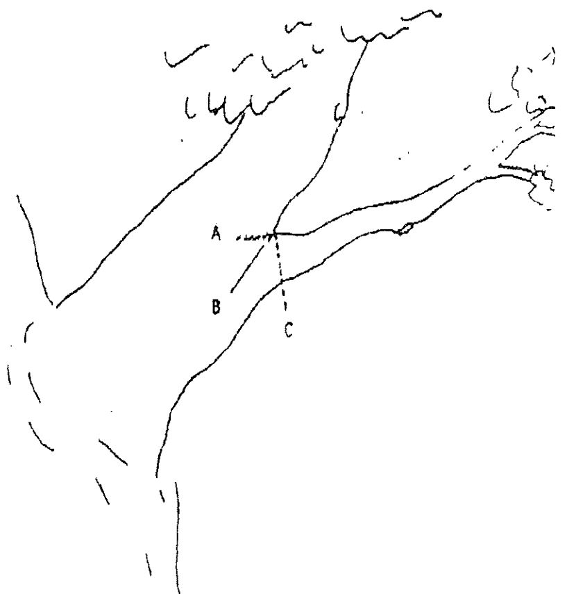
Figure 2. In removing a limb without a branch collar, the angle of the final cut to the branch bark ridge should approximate the angle the branch bark ridge forms with the limb. Angle AB should equal angle BC.
